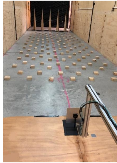
Figure 1: The experimental setup in the University of Adelaide wind tunnel. (a) Schematic of the setup, (b) photograph of the setup looking upstream from the plate.
